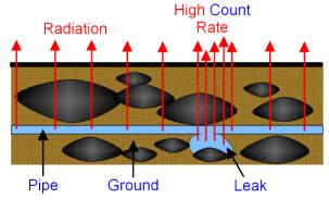
The isotope used for this purpose must be a gamma emitter, have a half-life of at least a couple of days (to allow for the leak to be found), and not be poisonous to humans who will drink the contaminated water.
